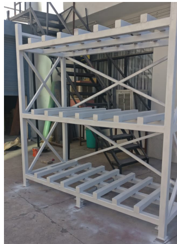
Die & Moulds Storage Rack
